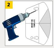
Drill 2 holes as indicated on the mounting template. Make a hole for the cable.
