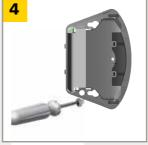
Position the sensor and fasten the screws firmly.
