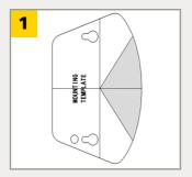
Use the adhesive mounting template to position the sensor correctly. The grey area indicates the measurement range.
